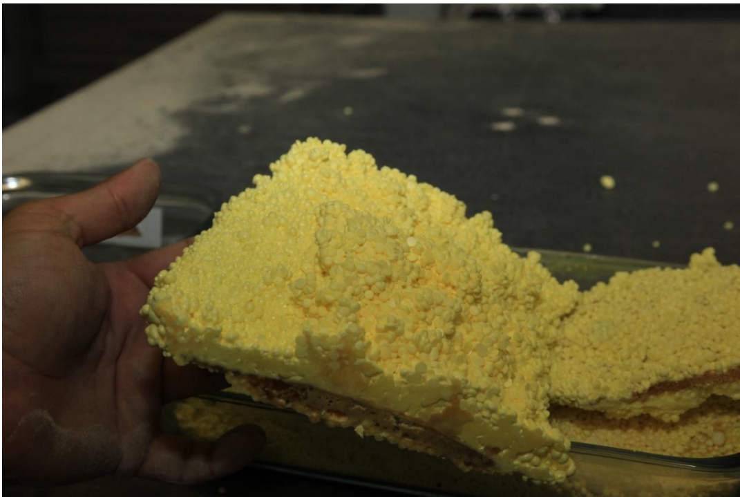
Photo #4 Fusing of melted sulphur. NOTE: Particles underneath remain intact.
